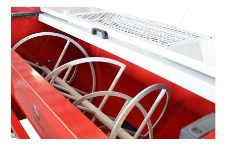
Compressed bales of peat moss or substrate are added to a bale breaker (or fluffer), many of which have ribbon blenders as seen in this picture. Run the breaker long enough to uniformly break up compressed substrate and then empty the machine quickly to avoid damage to the substrate structure.
