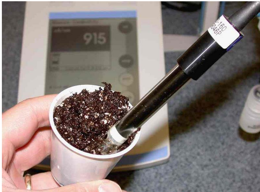
A combination E.C. and pH meter is used to measure these parameters of a growing medium sample. Source: Premier Tech
