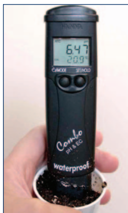
Frequent testing and recording allows you to verify the starting pH of unused growing medium.
