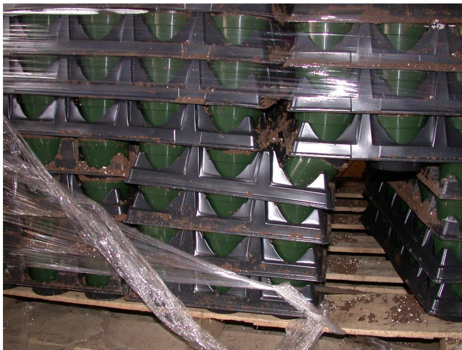
The trays holding containers in this picture have indentations on the bottom so that when stacked on other flats of filled containers they nest inside each other causing compaction. Notice the space between the flats is narrower on the bottom row vs the top row. Source: Premier Tech
