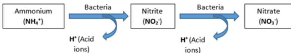
“Figure 2. Nitrification of ammonium into nitrate through soil bacteria.”
